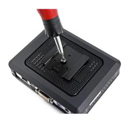
3 Insert the screws to secure the VESA bracket.
